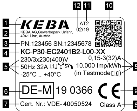
Fig. 4-7: Type plate (example)
